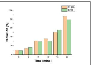
**Fig. 1.** Comparison between RLGA and XRD measurement in the afterglow (7 inches downstream from the core plasma). The particle temperature was  $1550\pm40~\rm K$ .
